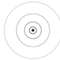
Beam shape of blur by "spherical aberration"
